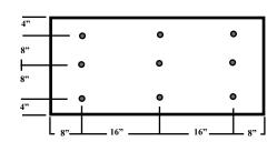
These suggested fastening patterns are typical for the attachment of EPS insulation used with EIFS PB Systems. Consult your EIFS Manufacturer for their particular requirements if different than above and for use in conjunction with adhesives.
