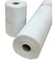
4.5 oz standard fiberglass reinforcing mesh made of multi-strand interwoven glass fibers. Fibers are coated with pigmented organic resin polymers to enhance their resistance to attack by alkalinity of mixtures containing Portland cements. Fibers will not rot, mildew or deteriorate. Ideal for strengthening or recoating stucco systems.
