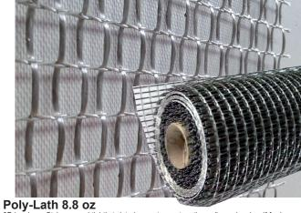
3D is a Leno Style weaved tightly twisted yarns to create a three dimensional, self-furring, open weave glass fibered lath. 1/4" Thick Poly-Glass fiber reinforcement lath is designed for use with traditional wall systems and cement applications. Self-Furring, Alkali Resist Lightweight, 31 lbs. per roll. Omni-directional, can be rolled out horizontally or vertically. Suggested Fasteners: 1-3/4" Anchor Plate with appropriate screw fastener
