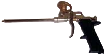
Economy Foam Gun The gun enables the user to adjust the product flow, thereby reducing waste. The gun is hermetically sealed, which prevents hardening of the product in the gun. Professional, metal, reusable gun. Nickel plated brass body. Barrel length 6" overall gun length 11", weight 1 lb. 2 oz.
