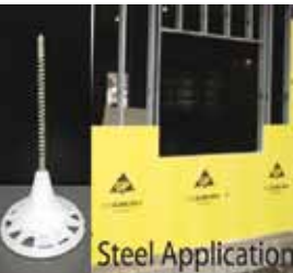
Steel Assembled Anchor III Plates with Exterior Coated Screw for EPS Insulation board through sheathing into steel studs. Self-Drilling from 20 ga. to 12 ga. Screw sizes do not allow for sheathing thickness.
