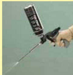
Remove adapter and attach can to gun basket to remove foam from gun barrel.
