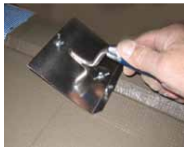
The Groove Tool with matching sled can also be used for smoothing out this joint with finish. Please note that the Square Grooves require a second plastic sled for the finishing of this groove. Included with the Groover Kits.
