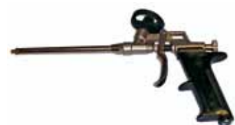
Teflon Foam Gun (Intermediate Series) The gun enables the user to adjust the product flow thereby reducing waste. The gun is hermetically sealed, which prevents hardening of the product in the gun. The basket has been coated with teflon for easy cleaning. Nickel plated brass body. Barrel length 6" overall gun length 11", weight 1 lb. 2 oz.
